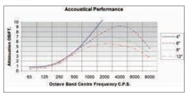
Material: Perforated aluminum core (min 25%) Thermal Resistance: R4.2, R6, R8 20.3 m/s (4000 fpm) Maximum Rated Velocity: Maximum Positive Pressure: 1.5 kPa (6 in. WC) Maximum Negative Pressure: 0.25 kPa (1 in. WC) -40°F to +250°F ( -40°C to +121°C ) Temperature Range: 1½ x diameter Bend Radius: Available Sizes: 4" to 24" Standard Lengths: 10ft ULC Listing: Class 1 Connector
